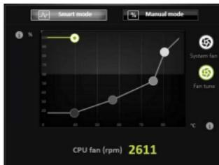
BIOS Hardware Monitor sub-menu allows you to set the temperature levels and the corresponding fan speed levels.
