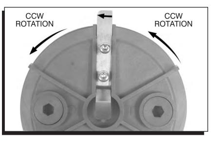
The reason for this modification is because voltage will travel to and from the sharpest point of the rotor tip. By rounding the leading edge of the Tip, the voltage will jump from the sharp point (trailing edge) of the tip which will be closer to the spark plug wire terminal when the timing is retarded. This will produce proper spark distribution even when the timing is retarded (which alters the rotor phasing).
