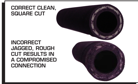
Figure 5 Severing the Hose Properly.
