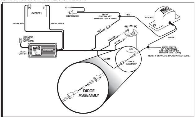
Figure 2 Wiring With the Diode Assembly.
