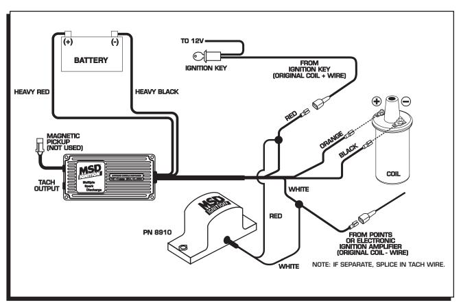
Figure 1 Wiring the Tach Adapter.
