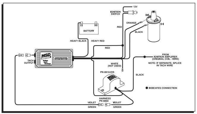
Figure 1 Wiring the Tach Adapter.
