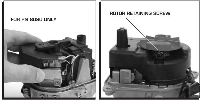
Figure 2 Removing Dust Cover
