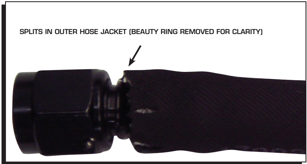
Figure 8 Improperly Installed Push-Lock Fitting
