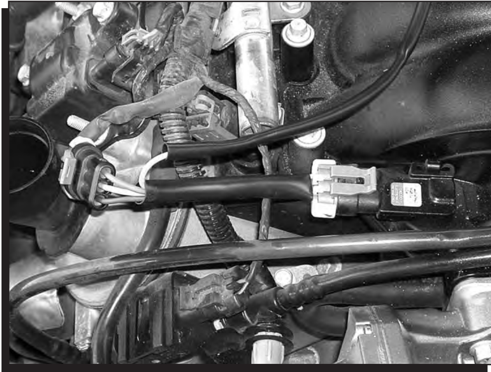
Figure 2 Map Sensor Connection.
