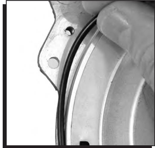
Figure 2 Installing the Distributor-to-Isolator Seal.
