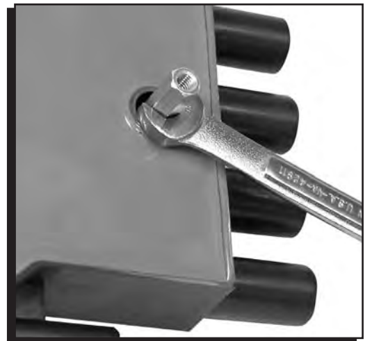
Figure 1 Removing the Original Cap.
