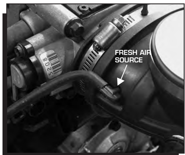
Figure 9 Installing the Fresh Air Line.
