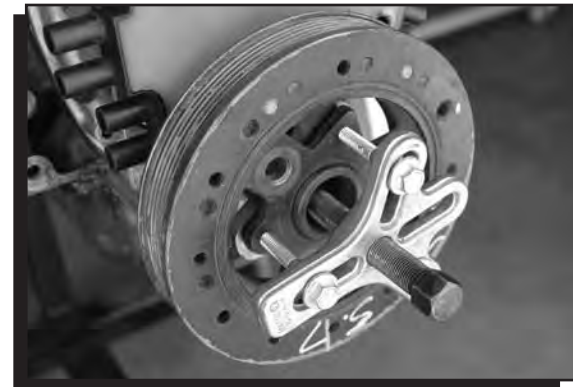
Figure 5 Removing the Hub.
