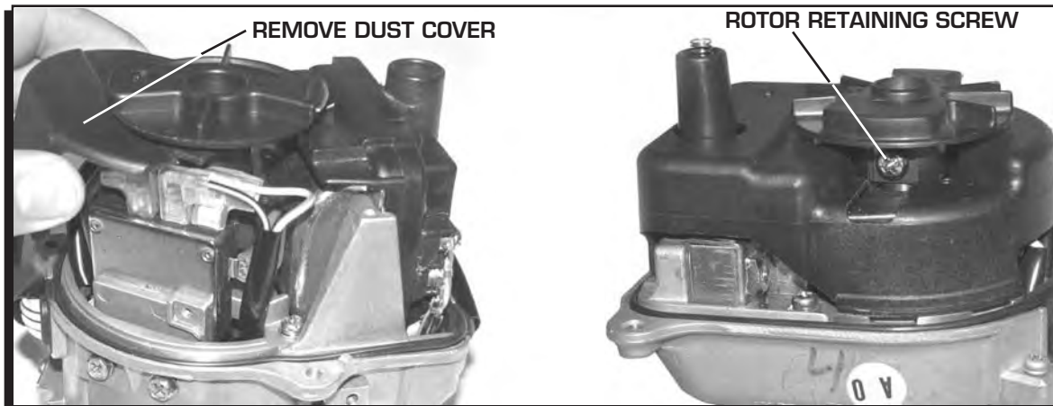
Figure 4 Replacing the Rotor.
