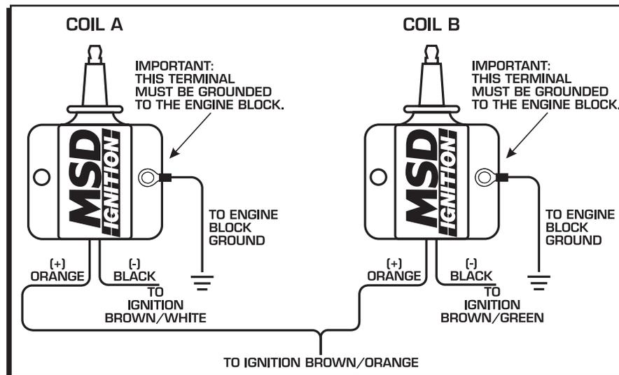
Figure 2 Dual Coil System to DIS-2 Ignition.
