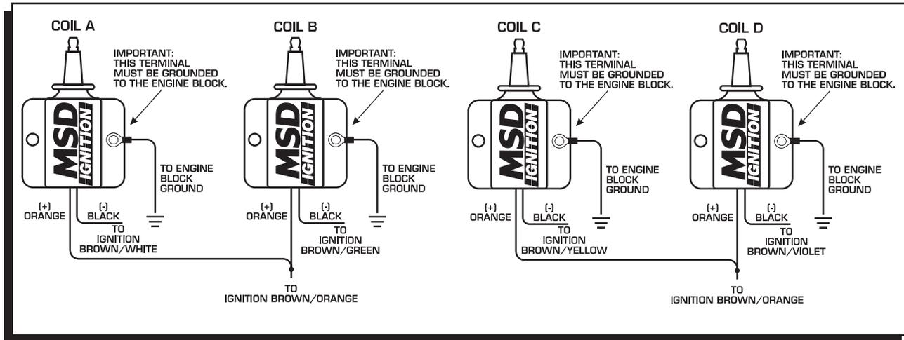
**Figure 3 Four Coil System to DIS-4 Ignition.**
