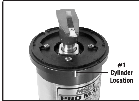
Figure 3 Positioning the Rotor Tip.
