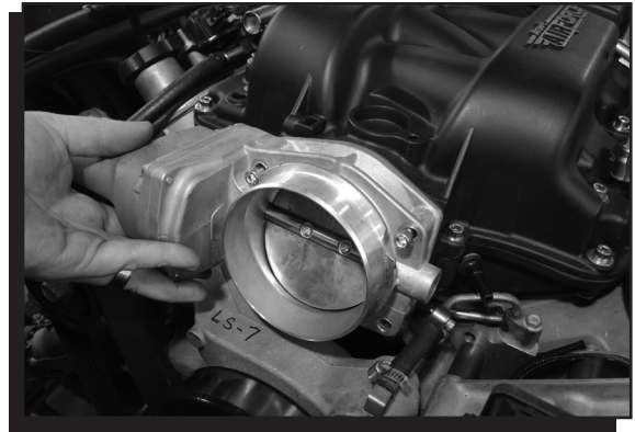
Figure 12 Installing the Throttle Body.
