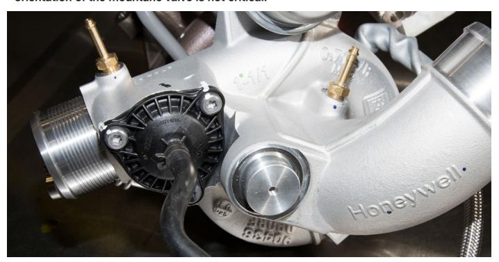
Step 2: Squeeze the clamp together holding the vaccum line to the OE re-circ valve.
