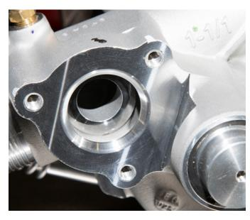
Step 5: Fit the mountune re-circ valve as shown - orientation of the valve is not critical.
