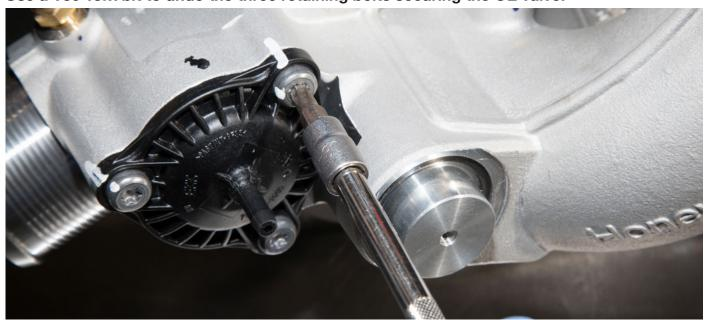
Step 4: The outer section of the valve will separate due to the spring, remove this, together with the rear section of the valve.
