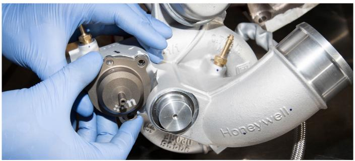
Step 6: Tighten the valve with the three Torx bolts removed previously. NB: DO NOT OVERTIGHTEN (2-3Nm)
