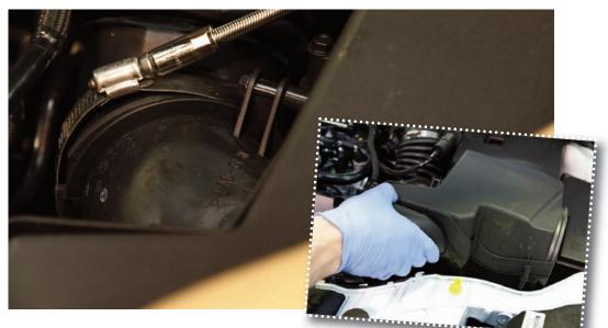
STEP 3A: (FOCUS) Separate the upper symposer pipe - it pulls off. - Go to STEP 5
