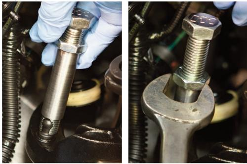
**STEP 7:** Slide the new billet shifter unit over the shifter arm. It can only fit one way and is an interference fit **NB:** Be aware some standard arms have flash which may need to be removed prior to installation.
