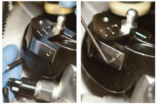
**STEP 9:** Push shifter cable end onto the new pin and check shifter engagement from the cabin. Re-fit airbox in reverse procedure to removal.
