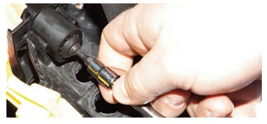
STEP 4B: (FIESTA) Separate the upper air feed by pulling the two pieces apart, then withdraw the airbox by pulling upwards - giving access to the shifter arm. **Go to STEP 5**
