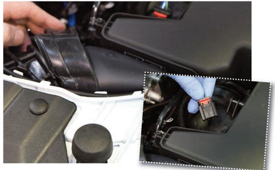
**STEP 2A:** Undo the convuluted hose to airbox clip and withdraw the airbox by pulling (FOCUS) upwards.
