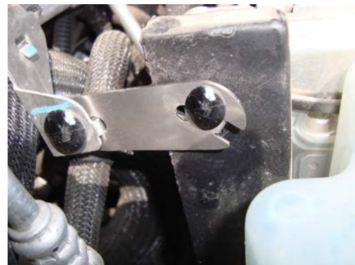
Move the smaller A/C line to the inside by removing push in keeper (re-use). Bend small tab on bracket down. Insert bent tab into original hole and push in new keeper.
