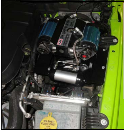
Stainless Steel Clips for 2015 models and newer. Used to move air conditioner hose towards the middle
