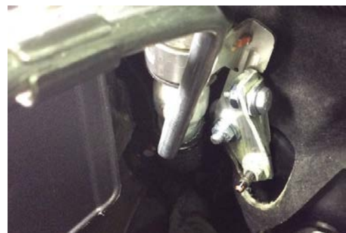
Modified location of Firewall bracket
