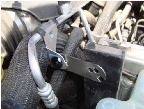
Move the smaller A/C line to the inside by removing push in keeper (re-use). Bend small tab on bracket down. Insert bent tab into original hole and push in new keeper.
