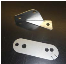
Stainless Steel Clips for 2015 models and newer. Used to move air conditioner hose towards the middle
