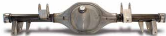
9" Bolt-In Impala Housing 1965-'70 and the 71-76 Impalas
