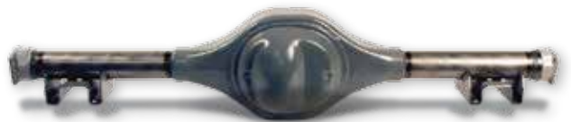
9" Bolt-In Housing - GM Mono-Leaf & Multi-Leaf 1962-67, 68-76 Nova, 1967-69, 70-81 Camaro
