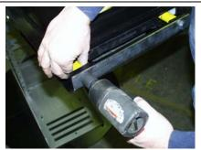
10) Tighten all 4 bolts and torque to 85 ft-lbs.
