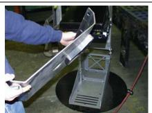
6) Slide Pull Rite skid pad (making sure wedge is to rear of box) into place.
