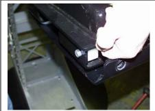
5) Install and tighten nut (self locker) x 4.
