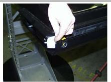
3) Slide spacer blocks into channel.
