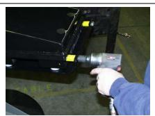
1) Remove four 9/16-12 bolts with 13/16 socket.
