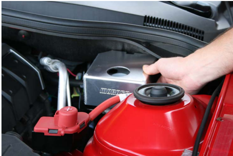
Step 4: Place cover over brake reservoir
