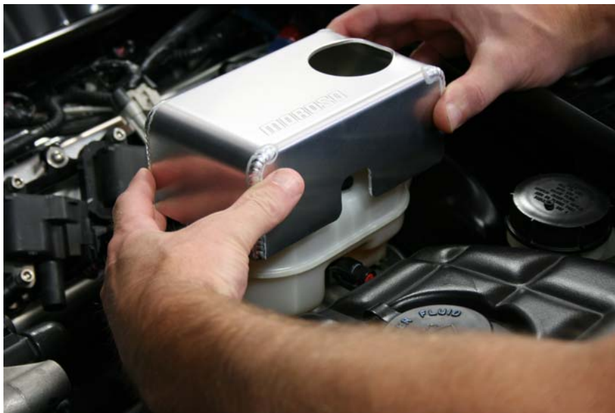
Step 4: Place cover over brake reservoir
