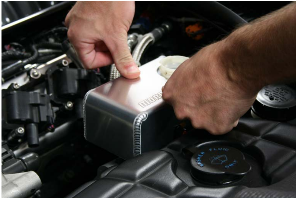
Step 5: Firmly press down on top of cover to seat Velcro dots-
