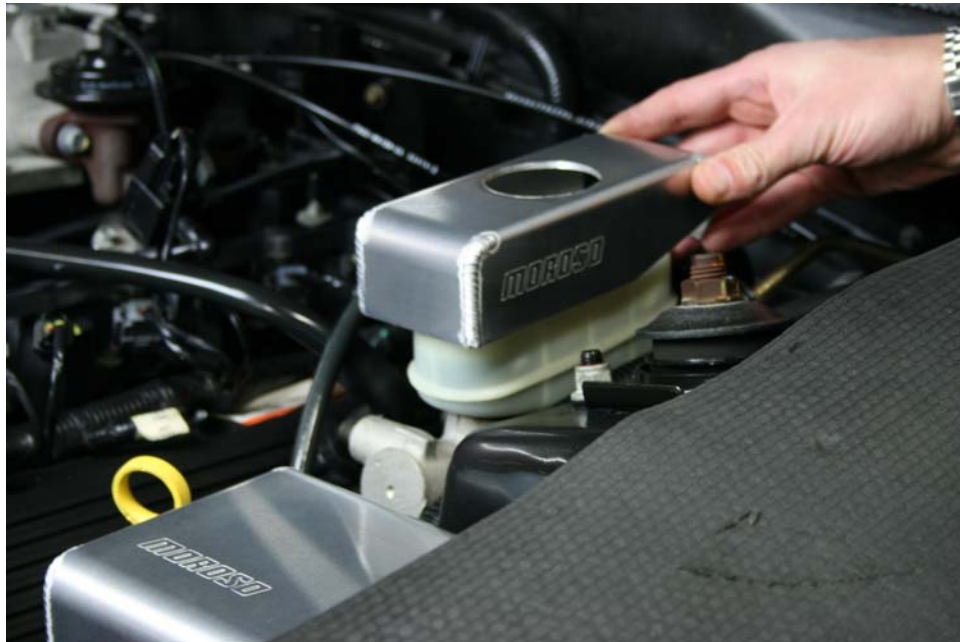
Step 3: Place cover over Brake reservoir
