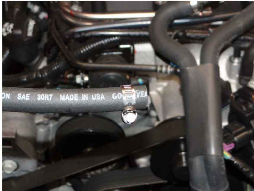
Step 3: Install hose clamp over 3/8 hose.
