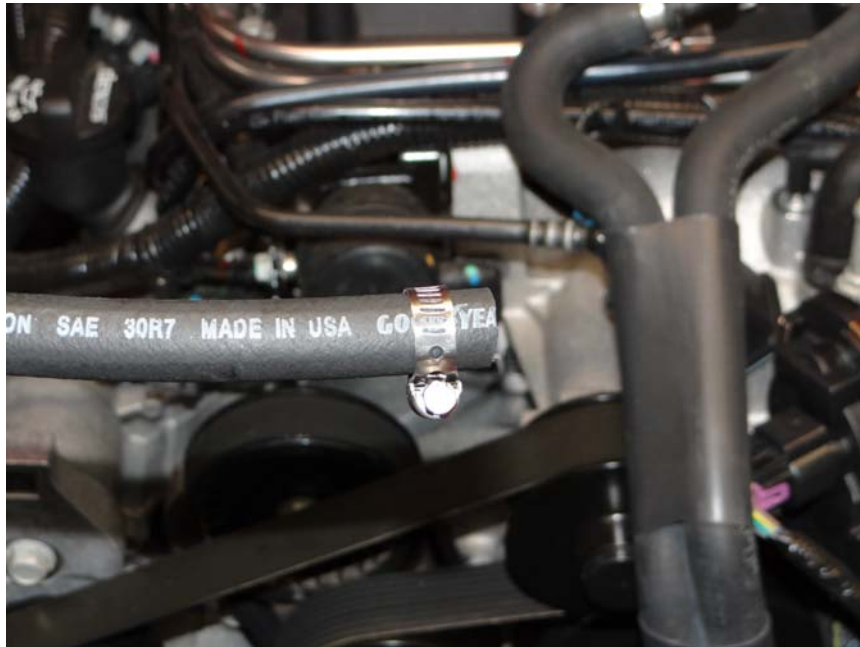
Step 6: Install hose clamp over 3/8 hose.
