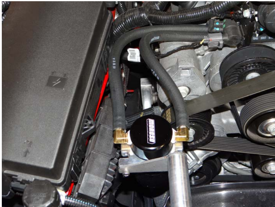
Step 11: Install 3/8 hoses to Air Oil Separator.
