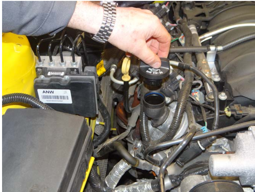
Step 2: Re-install oil fill cap.
