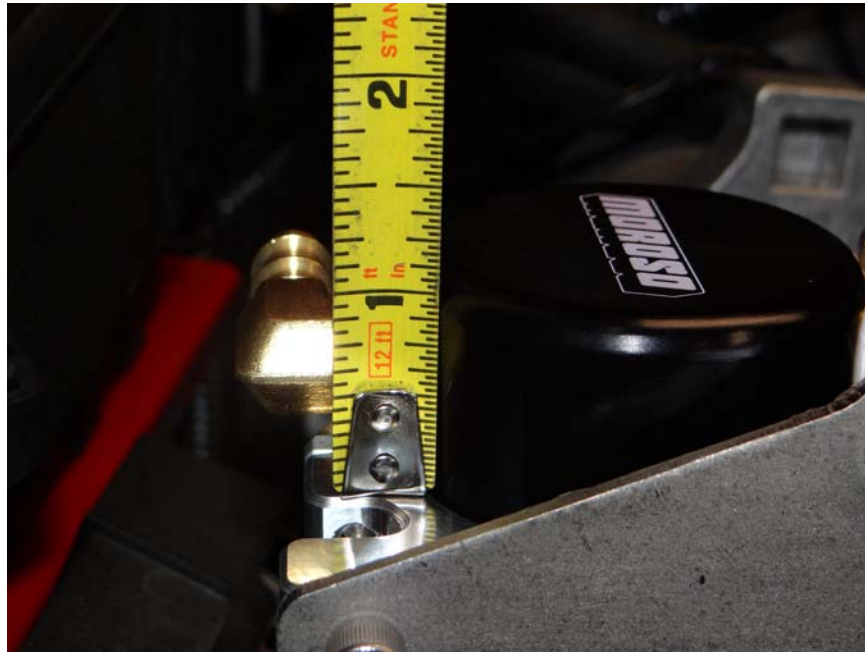
Step 10: Set Air Oil Separator to 1" as shown.
