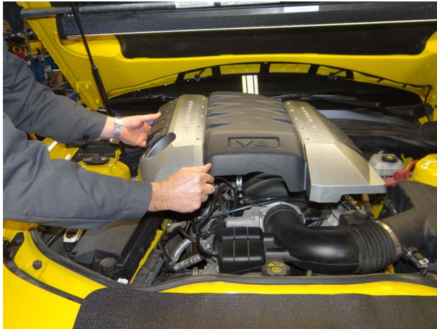
Step 1: Remove oil fill cap and engine cover.
