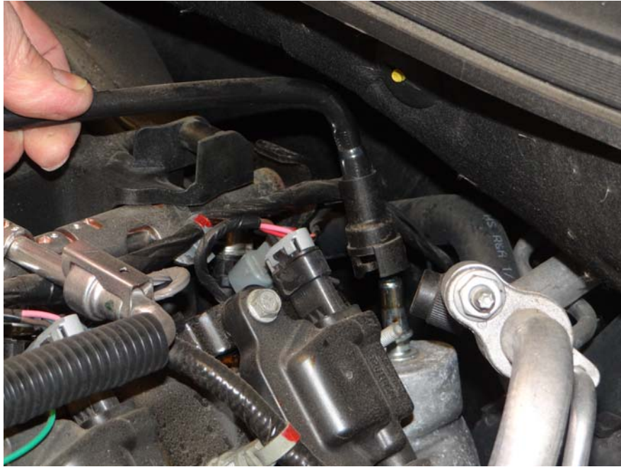
Step 4: Remove PCV line from valve cover.
