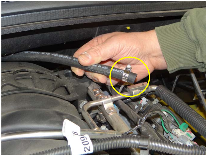
Step 8: Install hose clamp.
