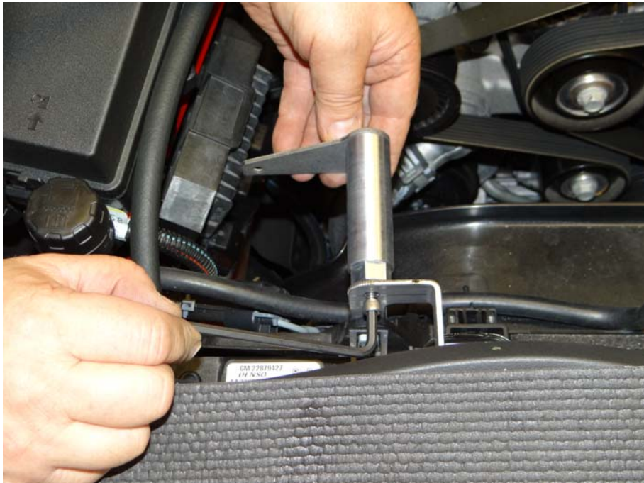
Step 5: Assemble to stainless steel mounting bracket as shown using (1) ¼-20 SHCS.
