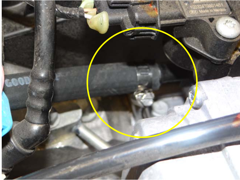
Step 12: Install hose over intake nipple.
