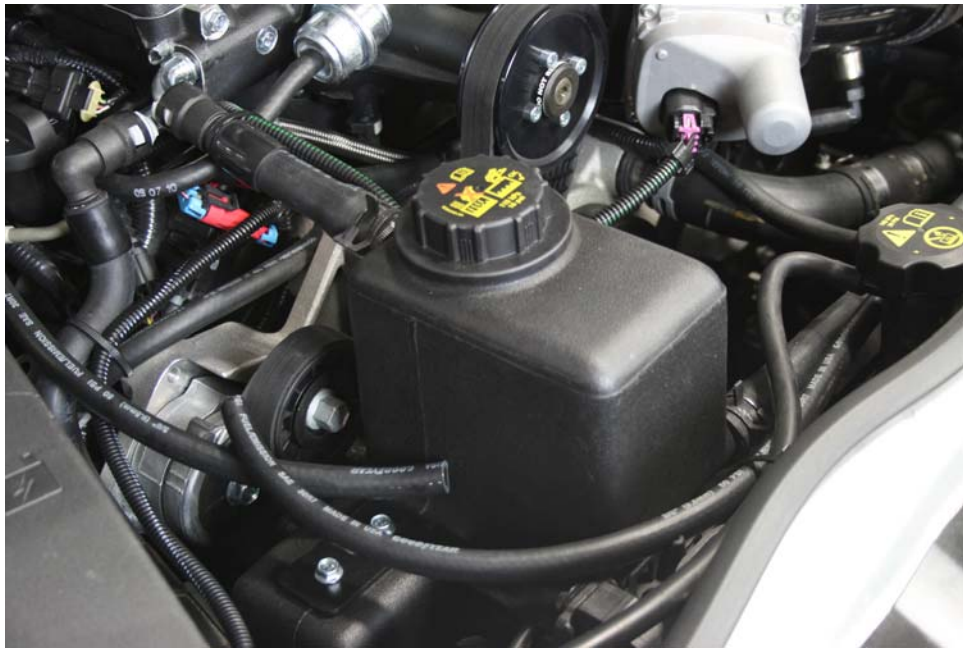
Step 8: Route hose as shown to other side of expansion tank.
