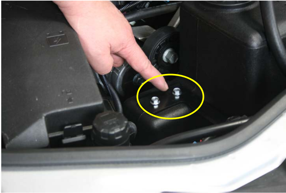
Step 12: Remove expansion tank mounting hardware
