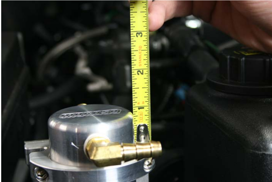
Step 15: Set height as shown from 1" to 1 1/8".
