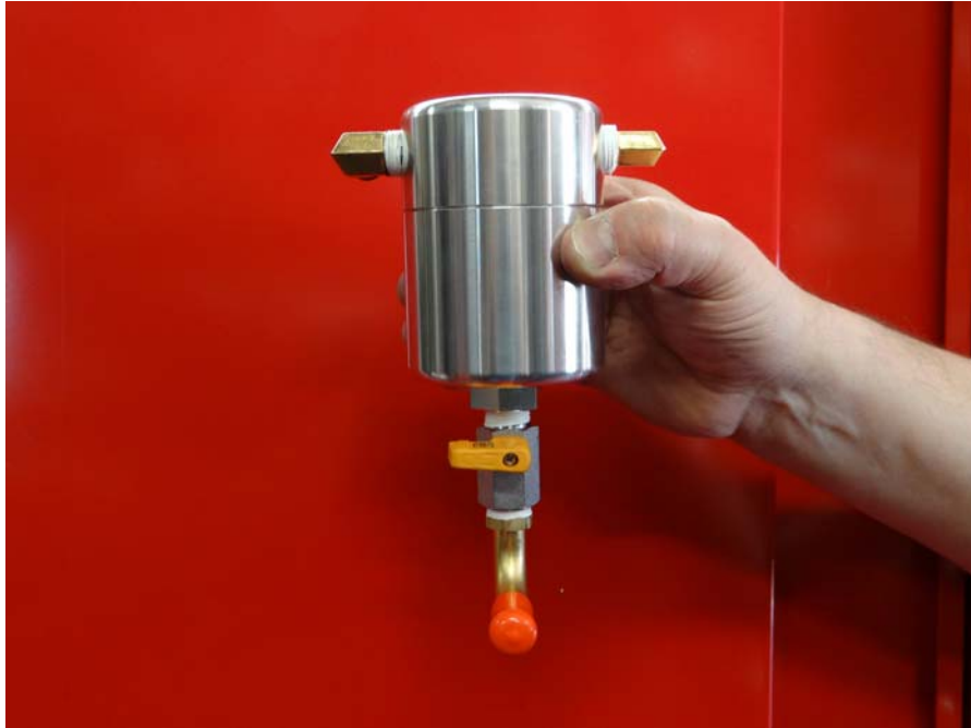
Step 11: Assemble Ball Valve, 90 degree Drain Tube and Drain Cap, using Teflon Tape on threads.
