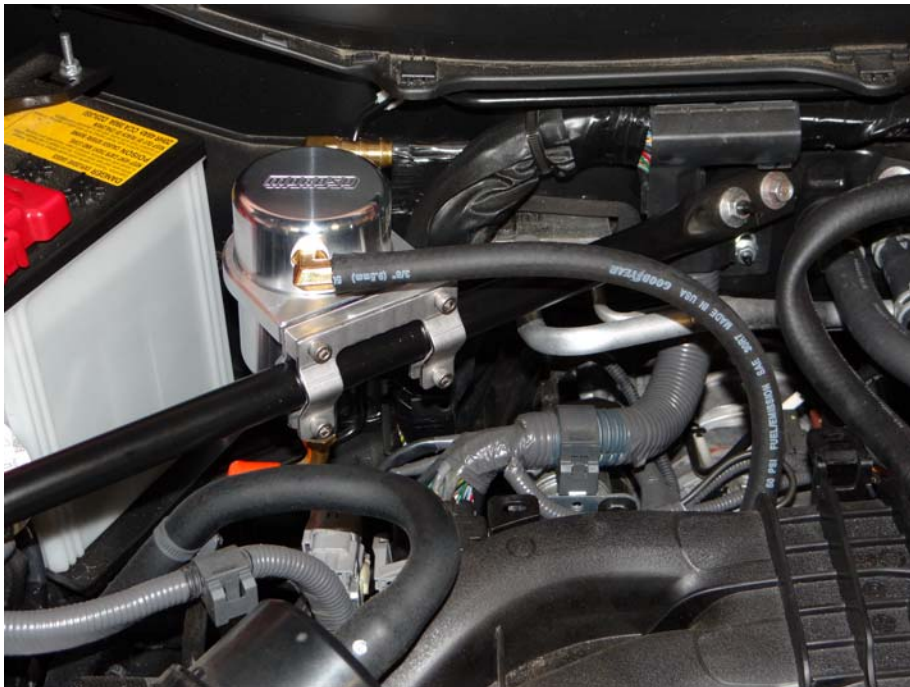
Step 14: Install 3/8" hose to 3/8" barbed fitting on Air Oil Separator.
