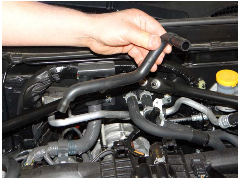
Step 4: Remove PCV line from PCV valve.
