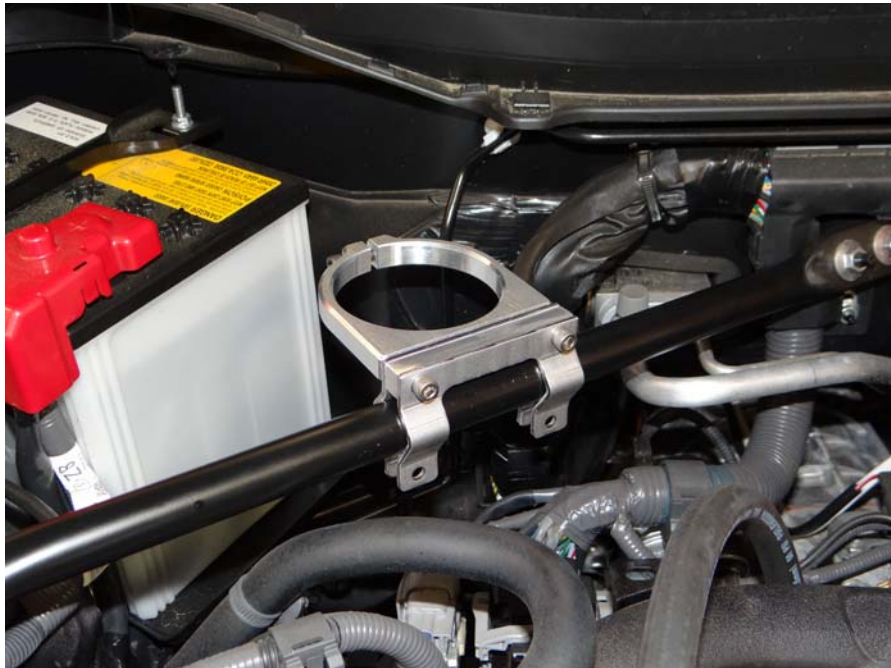
Step 8: Install mounting bracket to passenger's side strut brace as shown.
