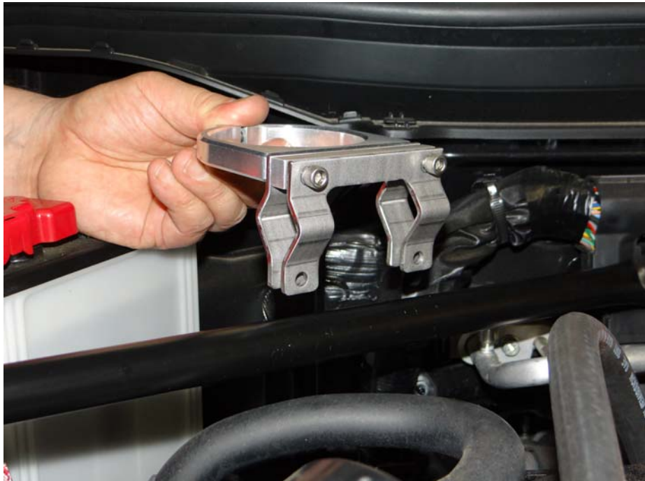
Step 8: Install mounting bracket to passenger's side strut brace as shown.
