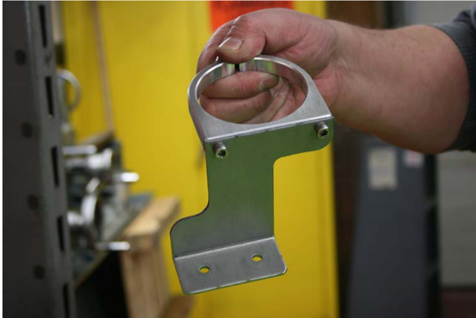
Step 11: Assemble billet clamp to stainless mounting bracket using (2) ¼-20x5/8 SHCS.
