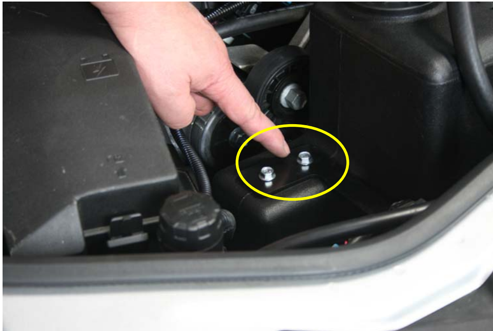
Step 12: Remove expansion tank mounting hardware
