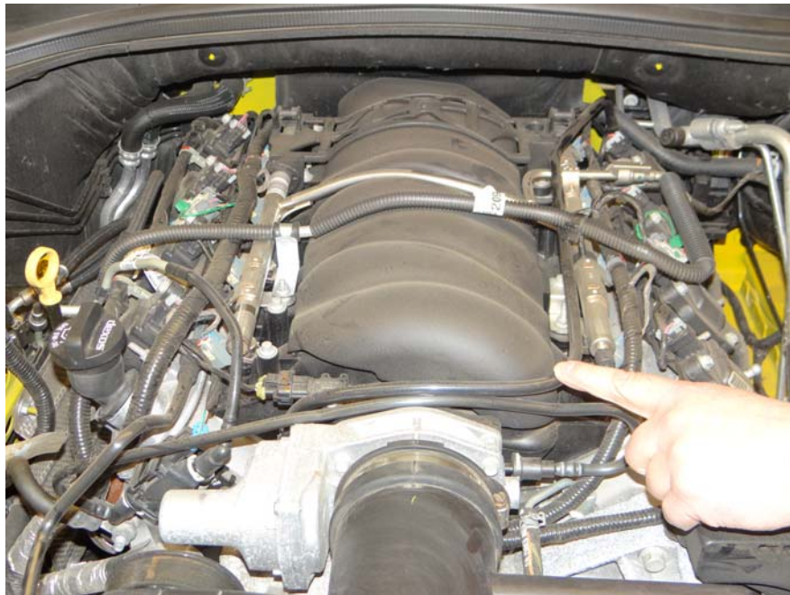
Step 3: Locate PCV line, runs from drivers side rear valve cover to intake manifold.
