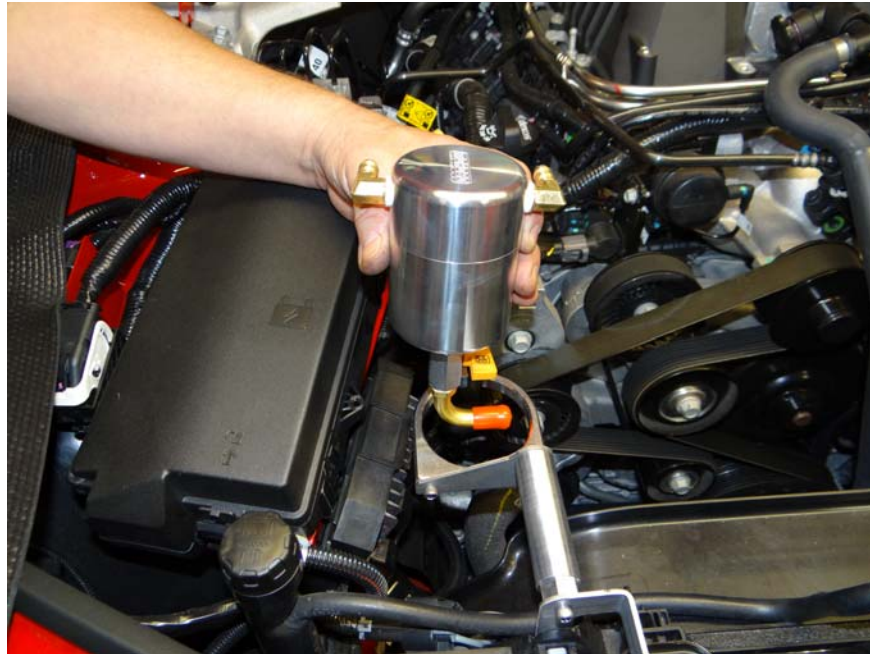
Step 9: Insert Air Oil Separator into billet clamp with barbed fittings facing firewall of vehicle.
