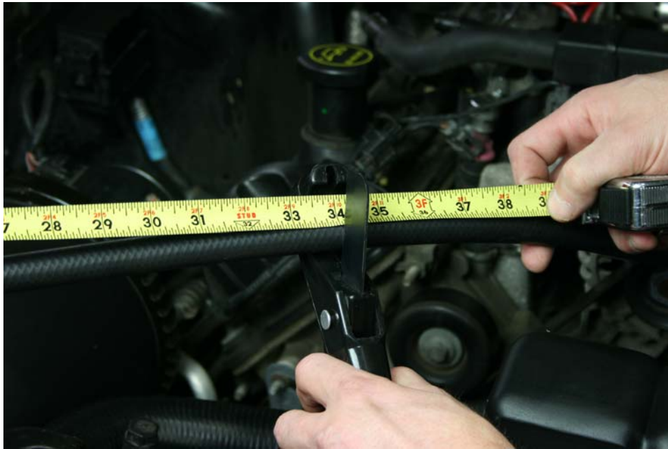
Step 14: cut 1 pc of 1/2" hose to 34"
