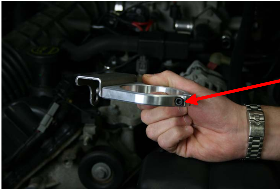
Step 10: Assemble Billet mount to Stainless Bracket as shown. Note orientation of 1/4" SHCS
