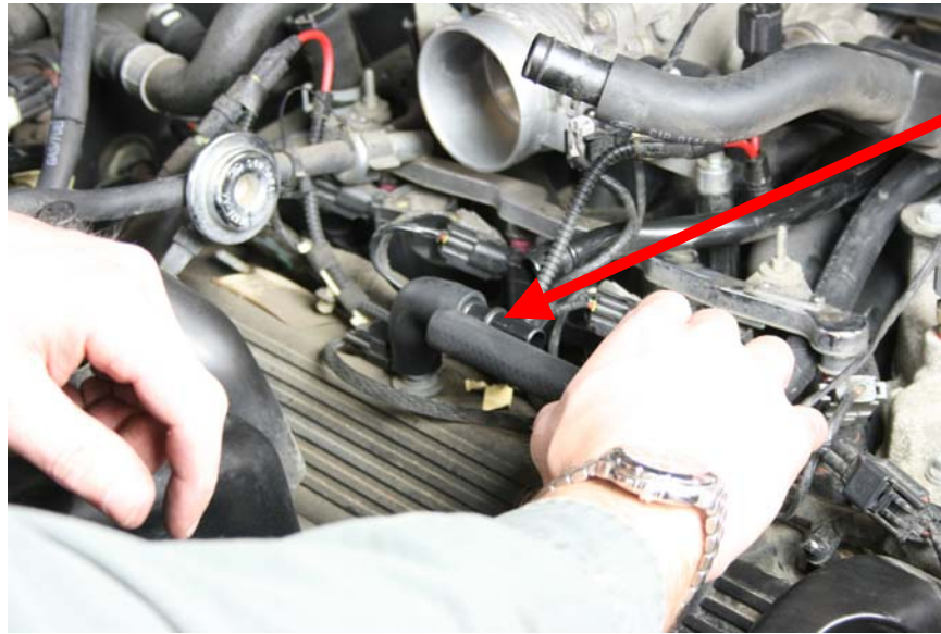
Step 18: Insert Nylon coupling into 90 degree fitting, install 90 degree fitting to PCV valve, trim 1/2" hose
