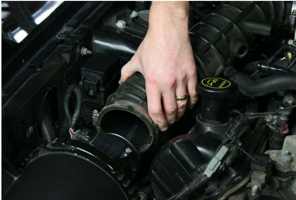
Step 4: Remove Air Intake hose from Air Cleaner Box, and remove from vehicle
