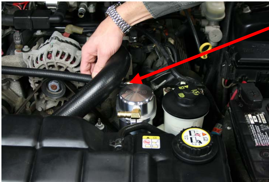
Step 15: Insert one end of 1/2" hose to rear fitting on Air Oil Separator
