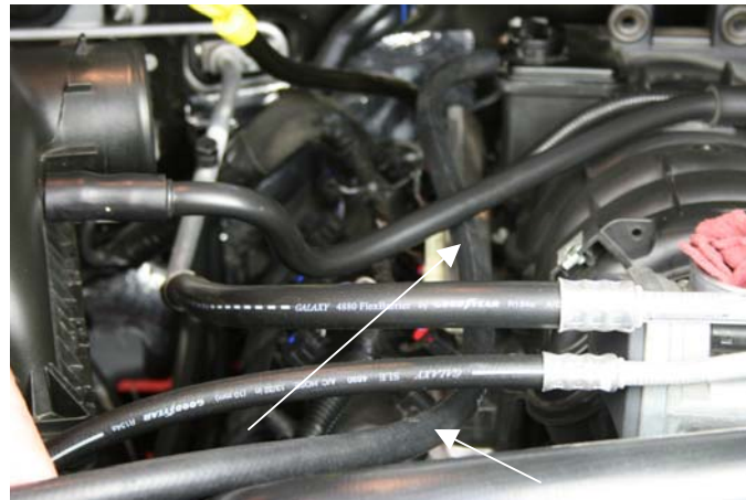
STEP 13 INSTALL 36" HOSE ROUTE AS SHOWN
