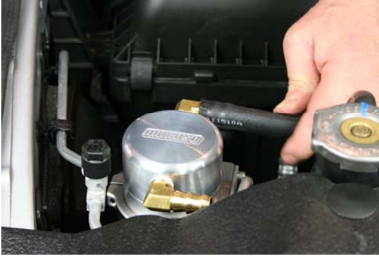
STEP 14 INSTALL 36" HOSE TO AIR OIL SEPARATOR
