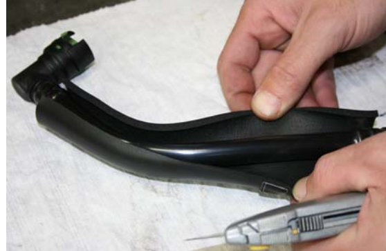
STEP 11 ADJUST CLAMP TO BODY TO APROX. 2"
