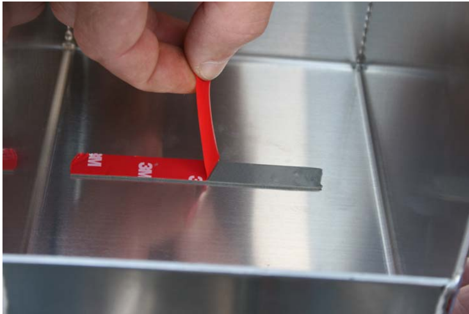
Step 3: Place double sided tape on inside of cover centered front to rear and side to side, peel backing as shown
