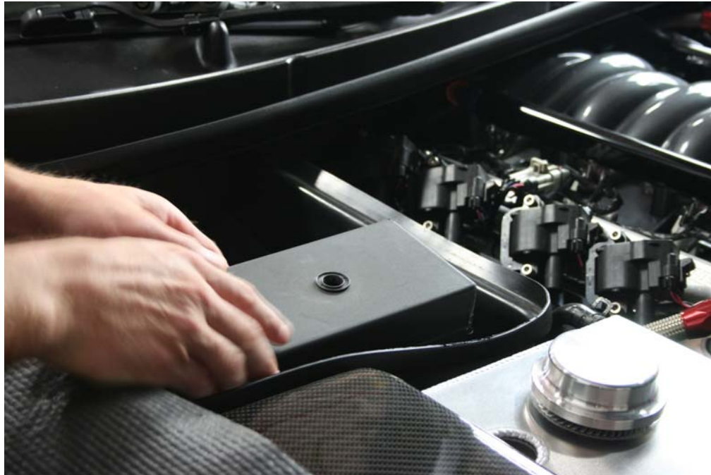
Step 7: Reinstall stock fuse box cover
