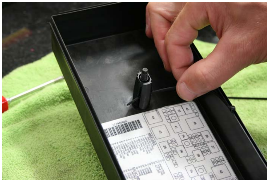
Step 3: Thread wire tie thru as shown in above
