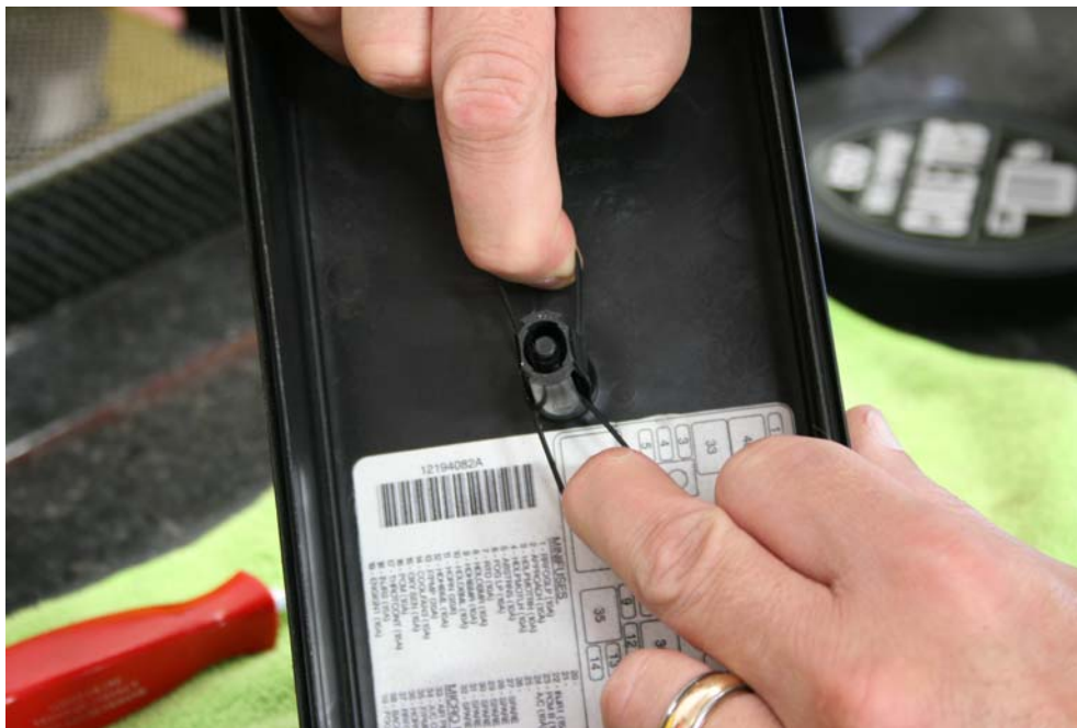
Step 5: Pull evenly on wire ties until mounting stud is released
