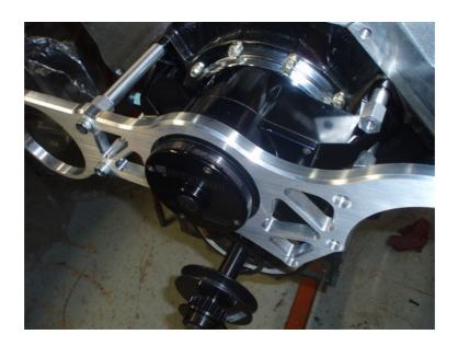
USING TWO 4.000" SOCKET CAPSCREWS, MOUNT THE OTHER SIDE OF THE BRACKET. PLACE THE SCREWS THROUGH THE BRACKET, THE TWO 2.700" SPACERS AND THE REAR ALTERNATOR SUPPORT AND THREAD THEM INTO THE SHORT, DRIVER'S SIDE STANDOFFS. DO NOT TIGHTEN THEM AT THIS TIME.
