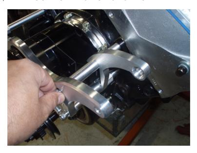
ONCE THE FOUR SOCKET CAPSCREWS ARE STARTED, GO BACK AND TIGHTEN THE FOUR STANDOFFS WITH A ¾" WRENCH. LEAVE THE FOUR CAPSCREWS FINGER-TIGHT UNTIL YOU HAVE THE ALTERNATOR MOUNTED.
