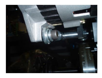
ONCE THE ADJUSTING LINK IS SECURED, THE DRIVE BELT CAN BE INSTALLED. TURN THE ADJUSTING LINK SO THAT IS AT IT'S SHORTEST LENGTH. WITH THE RECOMENDED 4.000 CRANK PULLEY (MOROSO PART#23523) INSTALL A 4L320 (32") V-BELT. ADJUST LINK TO ACHIEVE PROPER TENSION AND TIGHTEN BOTH JAM NUTS AND THE UPPER AND LOWER BOLTS.
