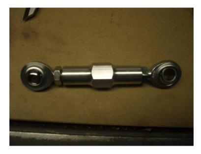
ATTACH ONE END OF THE ADJUSTER TO THE PLATE BY INSERTING A 3.750" SOCKET CAPSCREW THROUGH THE LOWER HOLE IN THE PLATE, THE .625" SPACER, ONE END OF THE ADJUSTING LINK, THE 1.450" SPACER AND THE REAR ALTERNATOR SUPPORT AS SHOWN BELOW. PLACE A FLAT WASHER AND 3/8 LOCKNUT ON THE END OF THE CAPSCREW AND LEAVE IT LOOSE FOR NOW.
