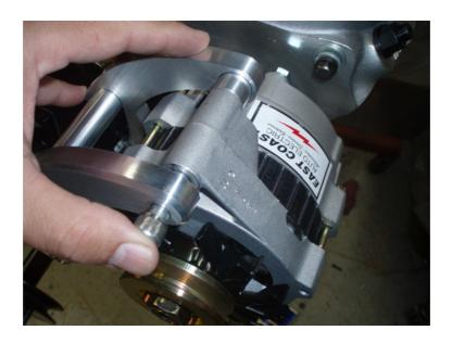
PLACE A 3/8" FLAT WASHER AND LOCK NUT ONTO THE ALTERNATOR BOLT AND LEAVE HAND-TIGHT. ONCE THE ALTERNATOR IS MOUNTED, USE A 5/16" ALLEN WRENCH AND TIGHTEN UP THE FOUR SOCKET CAPSCREWS THAT FASTEN THE MAIN BRACKET TO THE STANDOFFS.
