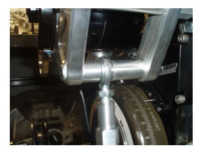
THE ALTERNATOR CAN NOW BE HUNG FROM THE UPPER MOUNTING HOLE IN THE MAIN BRACKET AS FOLLOWS. PLACE THE .590" SPACER INTO THE BORE OF THE REAR SUPPORT BRACKET AND HOLD IT THERE. WITH YOUR OTHER HAND, LIFT THE ALTERNATOR INTO POSITION BETWEEN THE BRACKETS, KEEPING THE SPACER IN PLACE. LET GO OF THE SPACER AND INSERT A 3.750 CAPSCREW THROUGH THE BRACKET, ALTERNATOR, SPACER AND REAR SUPPORT.
