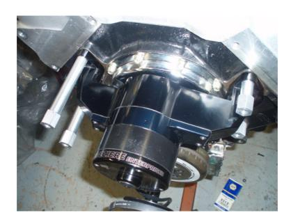
USING TWO 3/8 X 1.000" SOCKET CAPSCREWS, ATTACH THE MAIN BRACKET TO THE PASSENGER'S SIDE (LONG) STANDOFFS. DO NOT TIGHTEN AT THIS TIME, JUST START A COUPLE OF THREADS AND LET THE BRACKET HANG FOR NOW.
