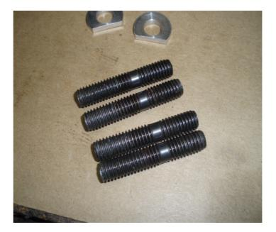
INSTALL THE GASKETS WITH SEALER AND SLIDE THE WATER PUMP OVER THE STUDS. PLACE THE FOUR "D"-SHAPED ALUMINUM WASHERS OVER THE STUDS WITH THE STRAIGHT EDGE FACING THE MACHINED RADIUS IN THE WATER PUMP FLANGE, AS SHOWN BELOW.
