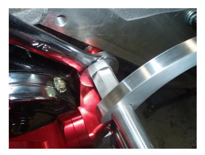
ASSEMBLE THE LOWER ADJUSTER BY THREADING THE JAM NUTS ONTO THE ROD ENDS, AND THEN THREADING THE ROD ENDS INTO THE ADJUSTING LINK.
