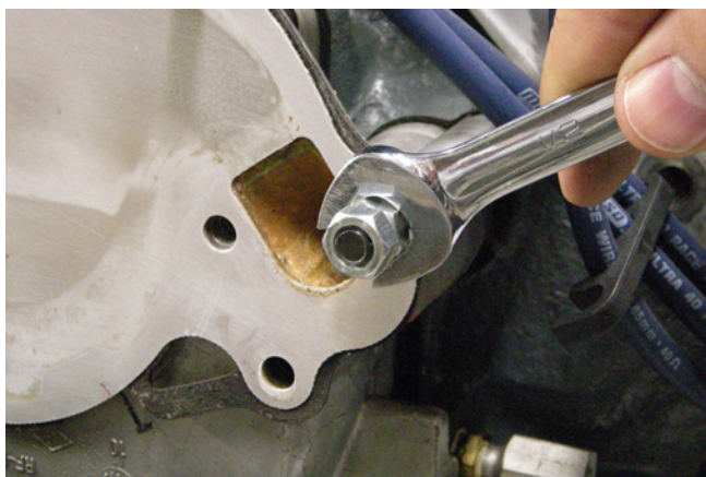
Long studs shown being installed in the water pump mounting holes, short threads in. Studs can be tightened by using the double-nut method
