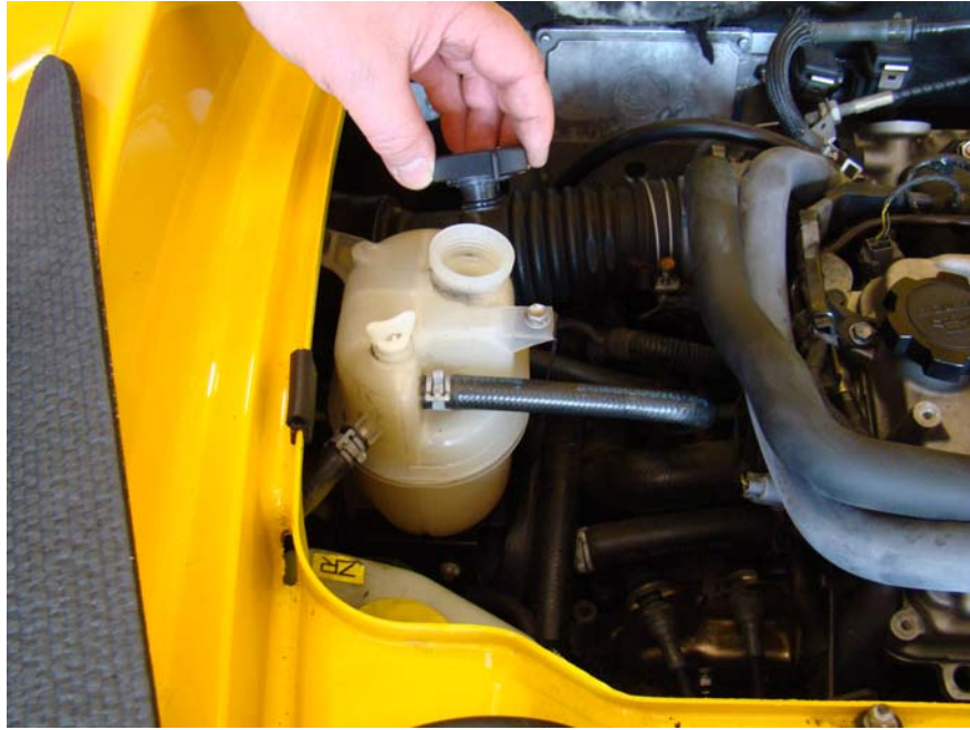
Step 1: Drain coolant tank
