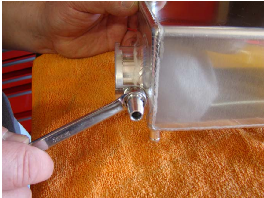
Step 9: Install and tighten overflow nipple using Teflon tape
