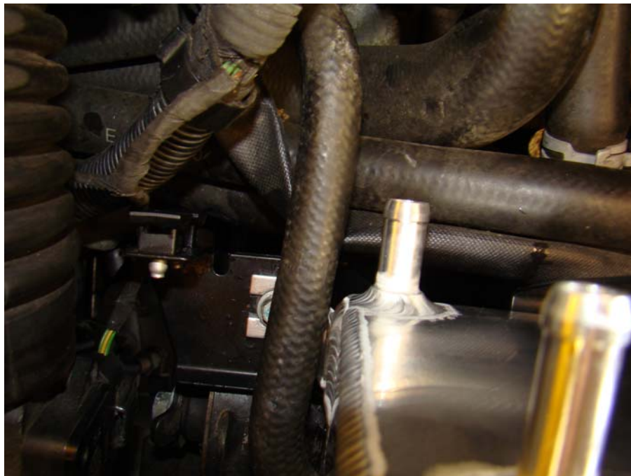
Step 21: Place line #3 next to tank as shown, mark desired length
