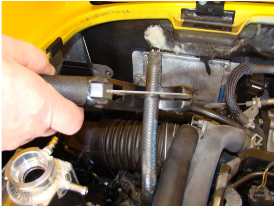
Step 25: Cut line #2 where previously marked
