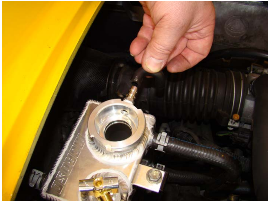
Step 28: Install overflow tube on overflow nipple
