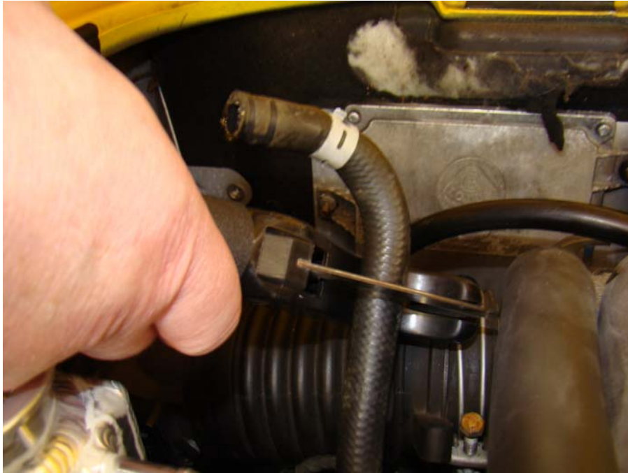
Step 22: Cut line #3 where previously marked
