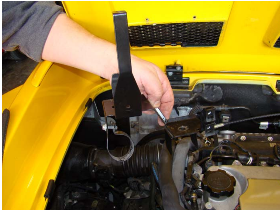
Step 8: Slide bracket over pump and remove from vehicle
