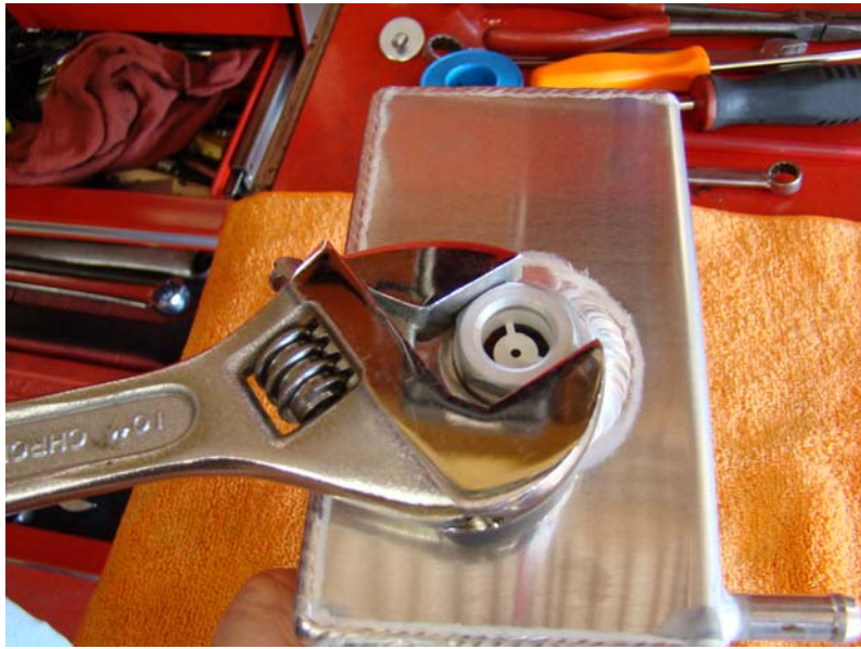
Step 11: Install and tighten sight glass
