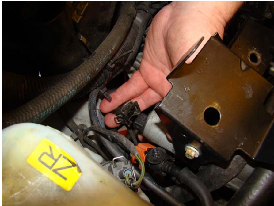
Step 7: Remove connector from pump
