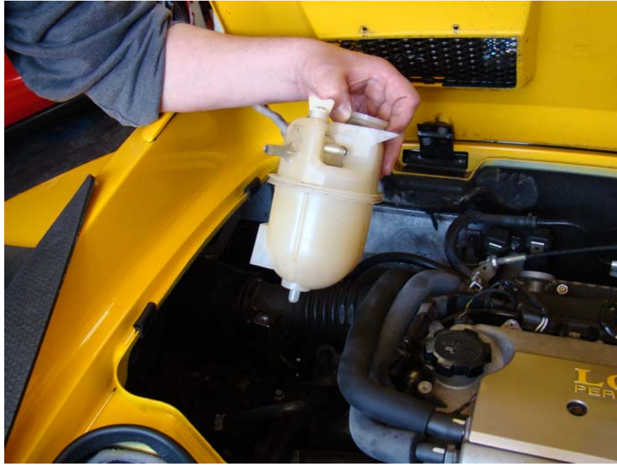
Step 4: Remove coolant tank from vehicle
