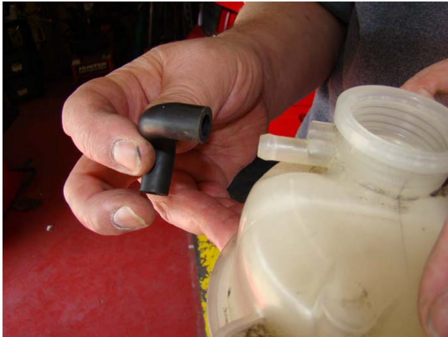
Step 27: Remove overflow tube from stock tank
