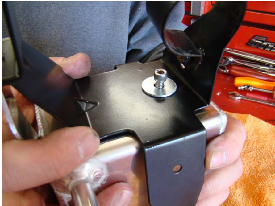
Step 13: Install 1/4-20 SHCS and fender washer on bottom of tank, do not tighten
