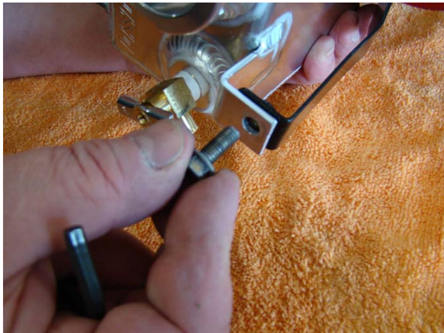
Step 14: Install stock mounting bolt in upper bracket, don not tighten
