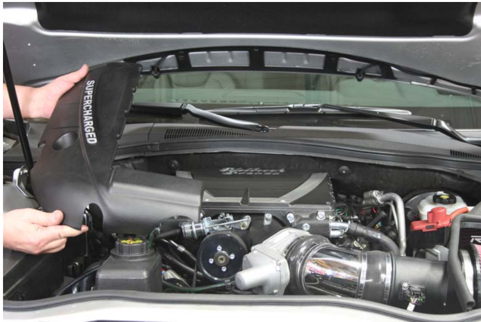
Step 1: Remove engine covers.
