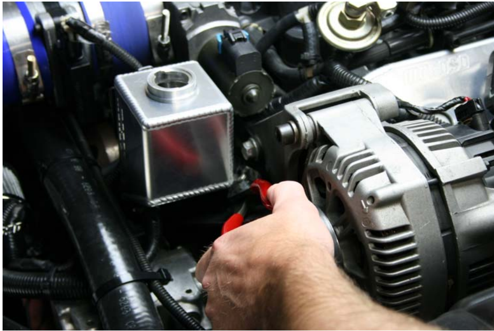
Step 10: Install rear line over nipple and reinstall hose clamp
