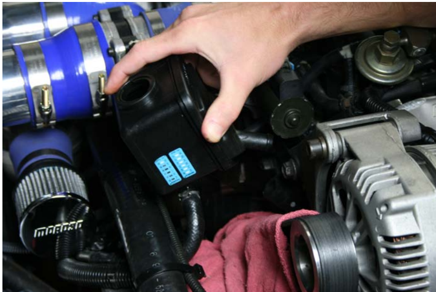
Step 4: Remove tank from mounting bracket and rear line
