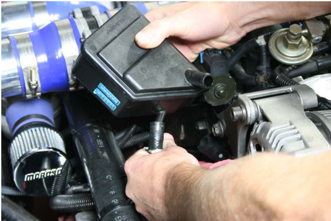
Step 6: Remove front line from tank
