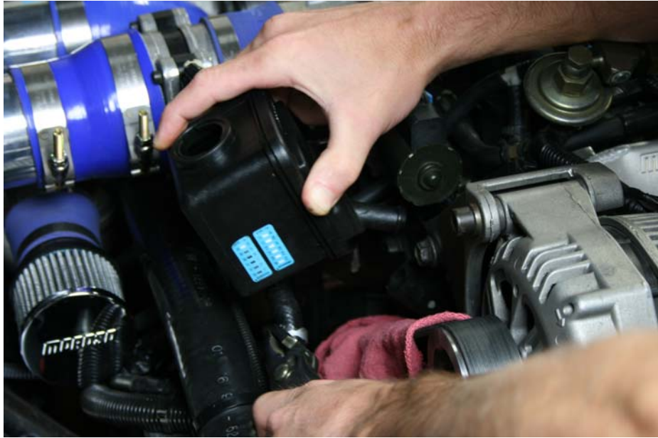
Step 5: Slide front hose clamp down from tank
