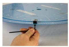
1-Attach the aluminum stands to the holes provided in the outer wheel. Insert the 10-32 screws into the deeper threaded hole while maintaining the flat side of the stand upward.
