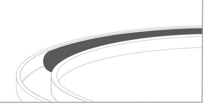
Use scissors to cut the Retro Rubber once the entire circumference of the housing has been filled.
