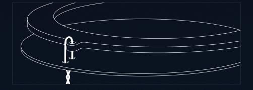
Place a bead of RetroRubber sealant in channel of headlight housing as shown. Fill the majority of the channel to ensure it sufficiently holds the front lens once re-installed.
