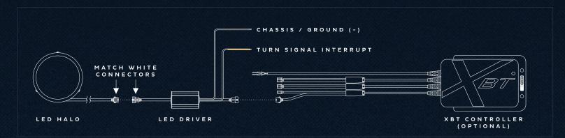
NOTE: The chassis / ground wire must be grounded to bare metal for the LED halo to function properly.
