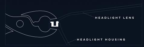
Allow thirty (30) minutes for headlight to sufficiently cool down prior to re-installation on car.
