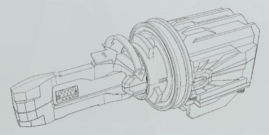
The proper alignment of the 2Stroke 3.0 bulb's LEDs is left and right, horizontally, as shown below. This alignment ensures the optical efficiency of the lamp assembly is fully retained.
