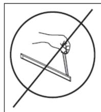
Do not pull tape liner prior to installation on vehicle.
