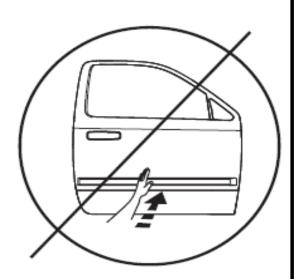
Vehicle Surface Temperature Do not pull tape liner prior to installation on vehicle.
