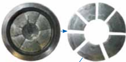
OTHER SUPPLIERS MAY USE AN OVER-STRESSED BELLEVILLE THAT SHATTERS AFTER CYCLIC LOADING, RESULTING IN EXCESSIVE LOOSENESS.
