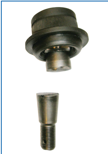
ALTERNATE SUPPLIER'S STUD, CRACKED DUE TO IMPROPER HEAT-TREATING
