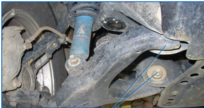
SEIZING OCCURS IN THESE AREAS, CAUSING ISSUES AND PREVENTING ALIGNMENT.
