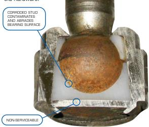
A failed OE part measured .025" of play, a result of the corroded stud wearing into the bearing surface.
