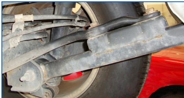
ORIGINAL DESIGN CAN LEAD TO INTERNAL CORROSION
