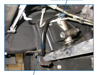
MOOG K6714 GREASE HOSE KIT WITH SKID PLATE REMOVED
