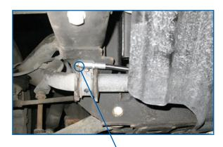
IDLER ARM BRACKET GREASE FITTING IS EASILY ACCESSIBLE THROUGH RIGHT FRONT WHEEL WELL WITH THE USE OF THE MOOG K6714 GREASE HOSE KIT.
